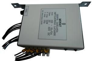
A photo of finished switched-mode power supply assembly for boom barrier lights type ZZI-01/24
